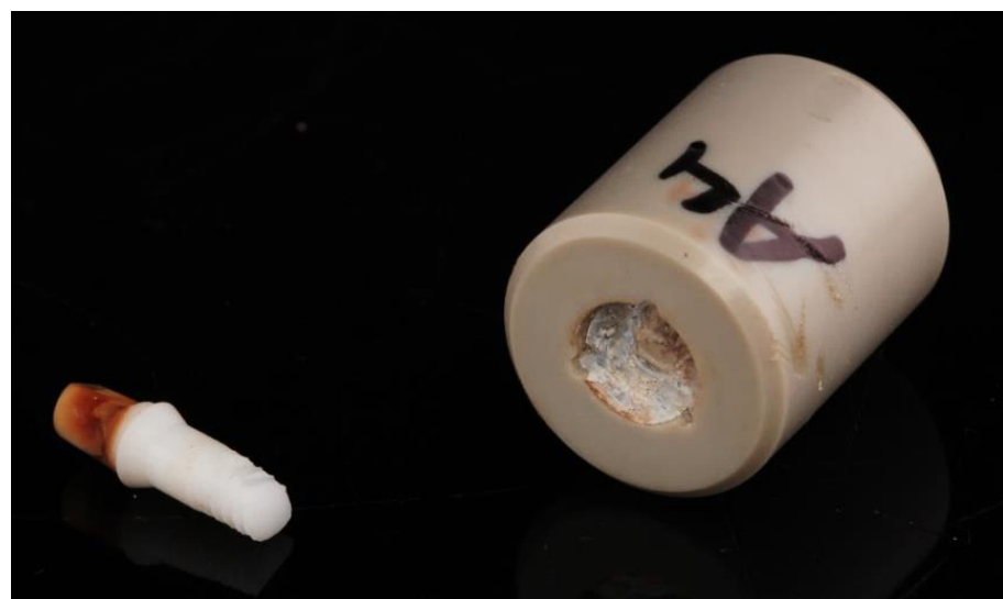
Figure 4. Fractured implant (DLHT4) after dynamic loading and hydrothermal aging. The fracture occurred inside the tube.
