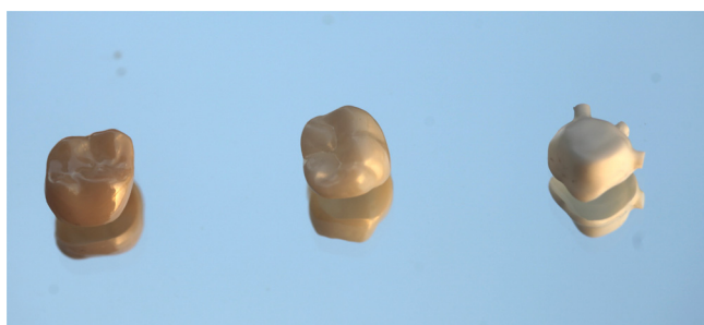
Fig. 5. A photo revealing the optical appearance difference among zirconia crowns with well-polished, self-glazed and blank-machined surfaces (from left to right).
