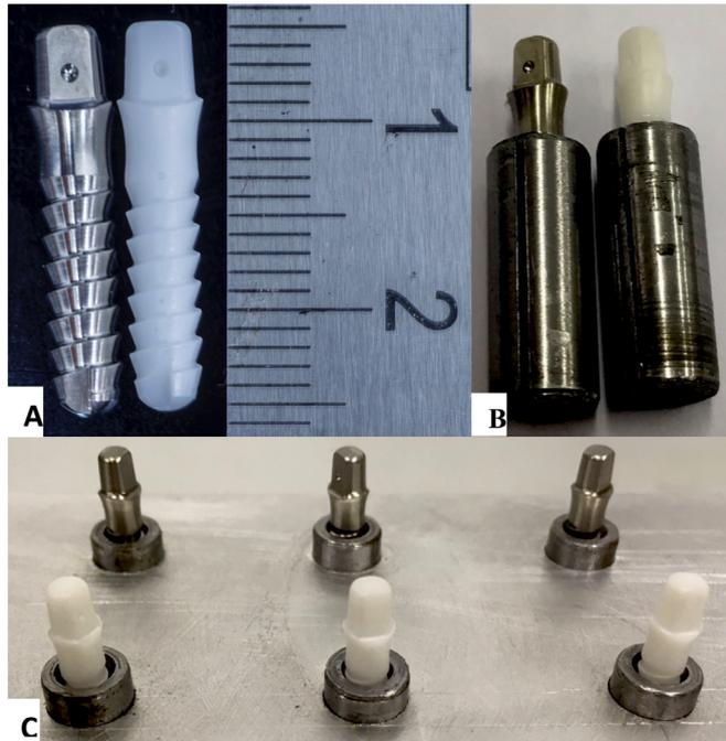
**Fig. 1.** A: Zirconia (right) and CP-Ti (left) implants. Note the geometrical similarity. B: Implants mounted in the steel sleeve. C: Gluing setup showing the first exposed thread.
