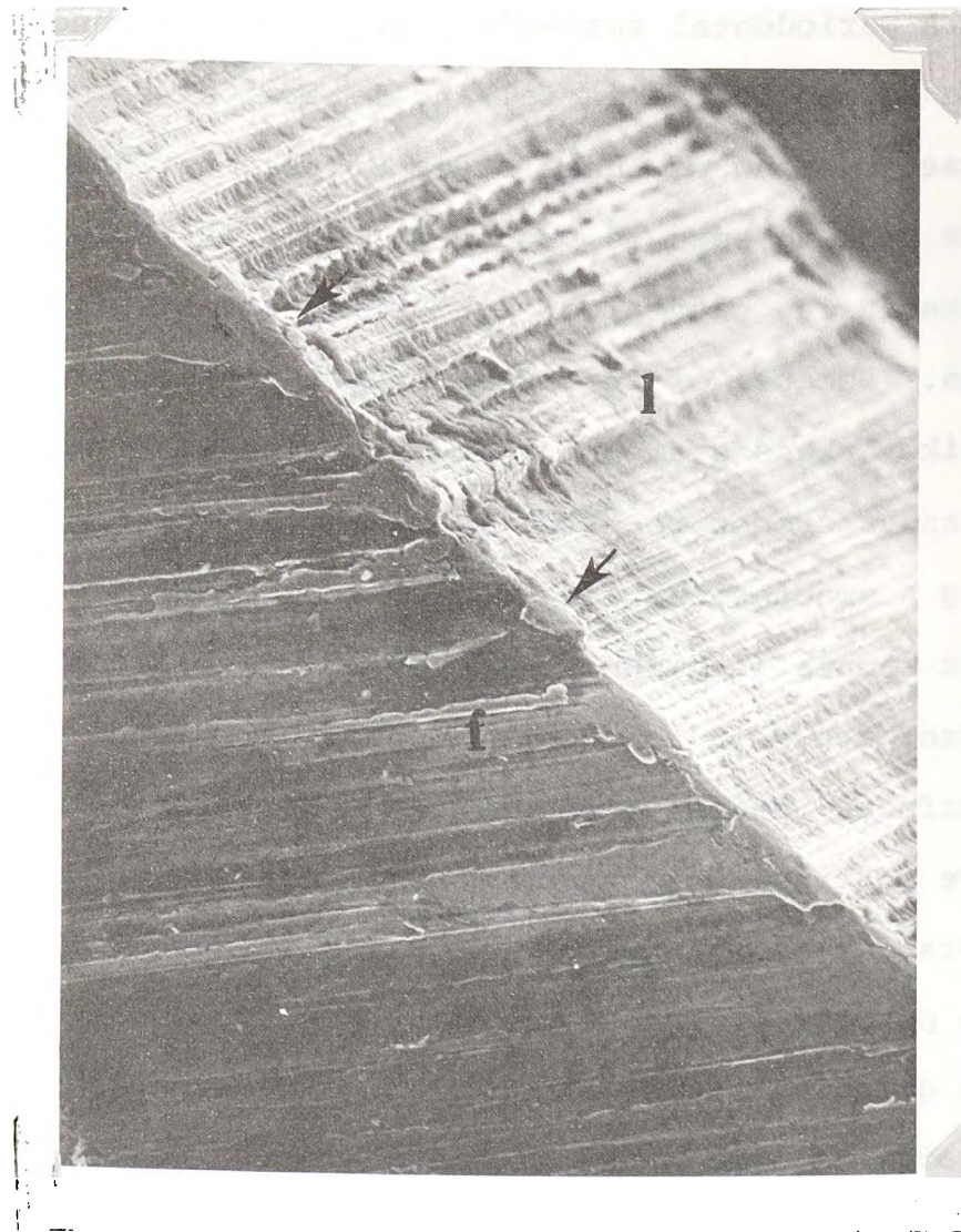
Figure 1A. Factory sharpened scaler. "f" is the facial surface and "l" marks the lateral surface. Arrows indicate the wire edges extending from the lateral surface. 500x.
